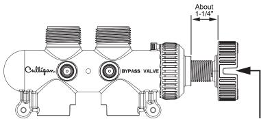
A screwdriver shank may be used in the slot as a lever for extra turning force if needed
